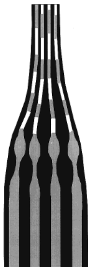
Figure 16. Schematic illustration of the fragmentation of the glassy PS lamellae during necking by deformation parallel to the lamellae. Gray scale: black, PB; gray, PS; white, void.
